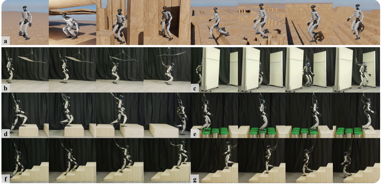
Figure 4. Humanoid robot traverses diverse 3D constrained terrains in both simulation and the real world. (a) Traversal across the eight simulated training terrain types. (b) Ducking under suspended ceiling obstacles. (c) Local navigation through lateral clutter. (d) Stepping onto a 30cm-high platform and crossing a 40cm gap. (e) Traversing pile-like stepping-stone terrain. (f)(g) Ascending and descending 20cm stairs. All deployments are based on the same policy .
